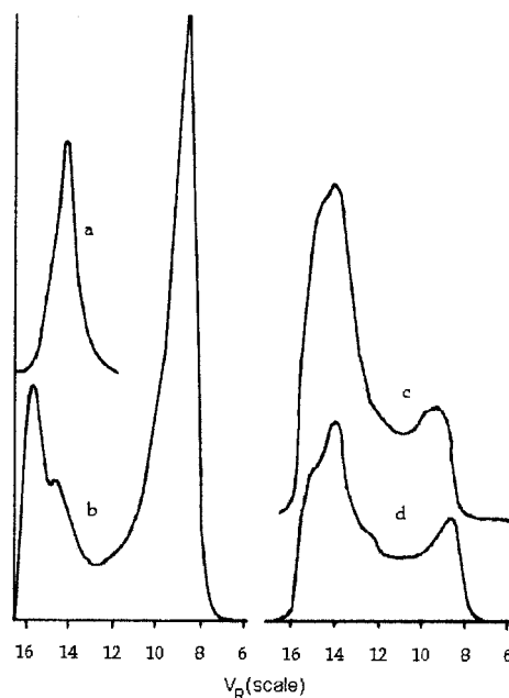
Figure 1 The molecular weight distribution curves of the condensation product of (a) OA, (b) OSA, (c) OSA-graft-OA-I, and (d) OSA-graft-OA-II.
